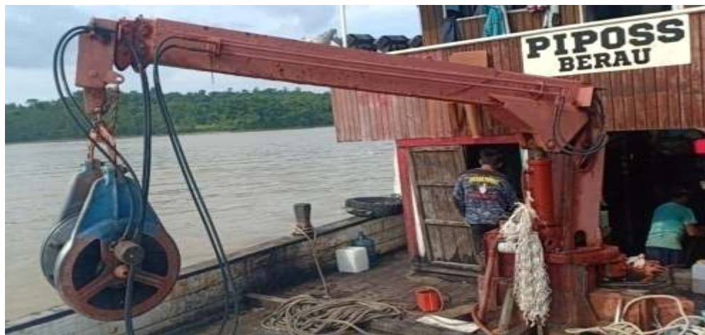
Gambar 2. Power Block KM. Piposs Berau
